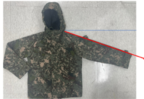
Fig. 5. Upper garment part of the developed NBC protective clothing.
