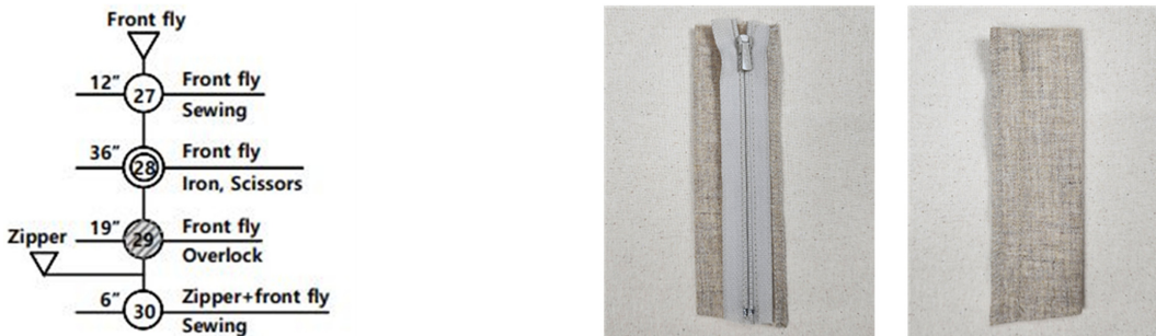
Fig. 12. Physical slacks front fly sewing process.
