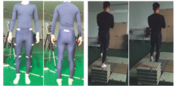
Fig. 2. Single-leg drop landing from 40cm height with three trials. (Lee et al., 2016)
