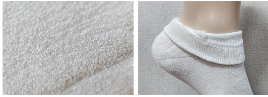
Fig. 7. Terry (ring) tissue close-up shot (left), sock neck knitted with B type equipment (right).
