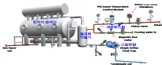
Fig. 14. Schematic diagrams of dyeing process by steam. KTTA (2023), p.18
