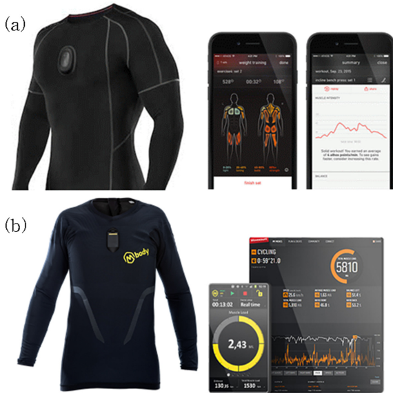
Fig. 1. Representative examples of EMG measuring clothing; (a) Athos shirt, www.liveathos.com , (b) Mshirt, www.myontec.com .
