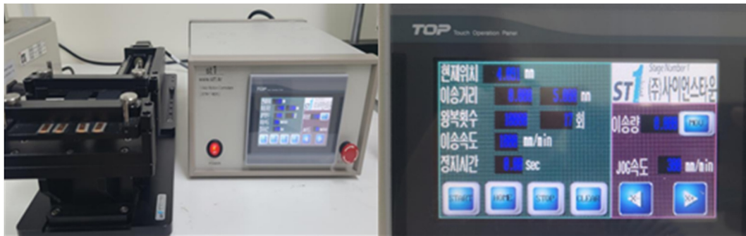
Fig. 4. Ten thousand times of stretching test of strain sensor.
