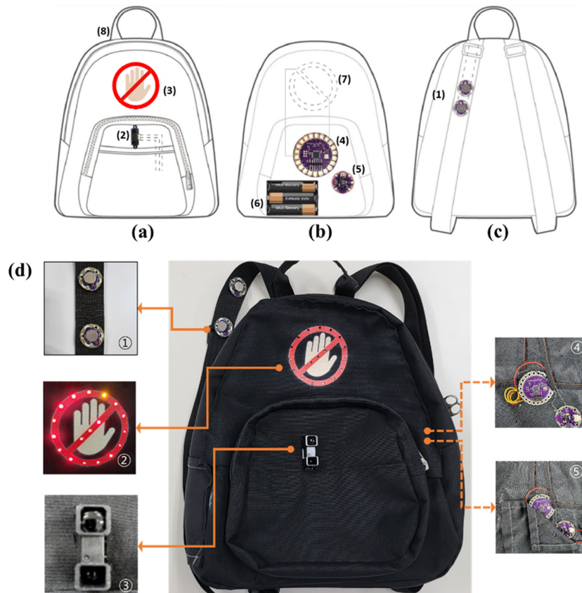
Fig. 7. Schematic illustrations: (a) front view, (b) inner parts, (c) vibration motors, and (d) prototype of the smart backpack system.
