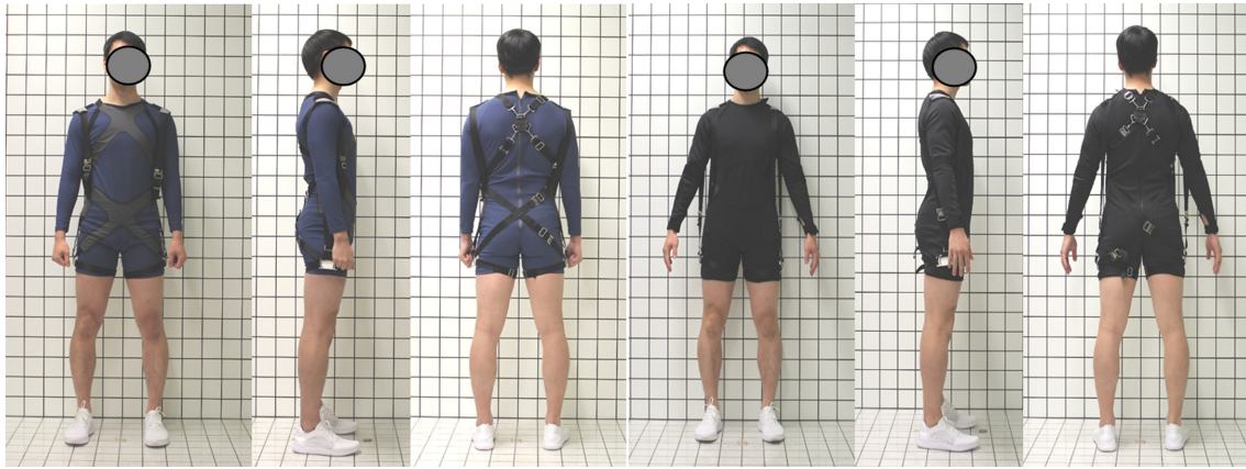
Fig. 6. Wear test of upper limb assistive wearable softrobot (left: 1st prototype, right: 2nd prototype).
