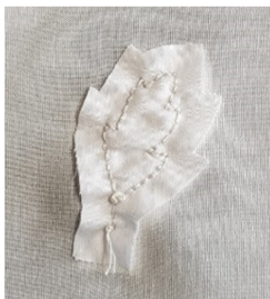
Image 4. After sewing, cut the top two cotton fabrics and the bottom two cotton fabrics with only 5mm remaining at the edge of the stitch.
