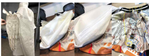
Fig. 8. Muslin basting and system circuit making and testing process of air-bag jacket (May 28th 2018).
