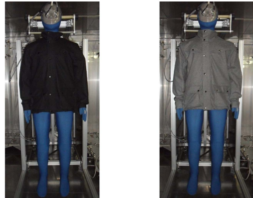
(a) Wool 100% specimen (b) Wool 50%/nylon 50% specimen Fig. 2. Images of thermal manikin experiment.
