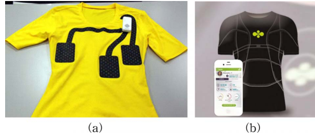
Fig. 2. Example of the smart clothing for ECG monitoring. (a) http://bizmakoto.jp , (b) http://nownews.seoul.co.kr
