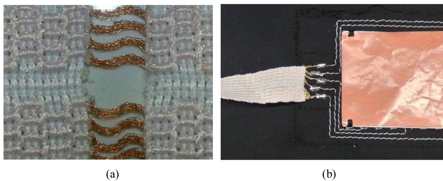
Fig. 5. Textile band for transmission: (a) textile band after skinning by using CO 2 laser system (b) soldered interconnection between textile switch and textile band.
